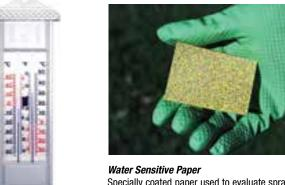
Specially coated paper used to evaluate spray droplet density and distribution as well as penetration of spray into the canopy of plants.
